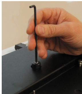
Figure 3-6: Opening the port with the hex wrench.
