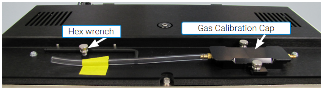
Figure 3-2: Hex wrench and gas calibration cap location.
