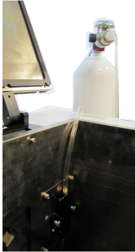
Figure 3-1: Using a Calibration Gas is the recommended method.
